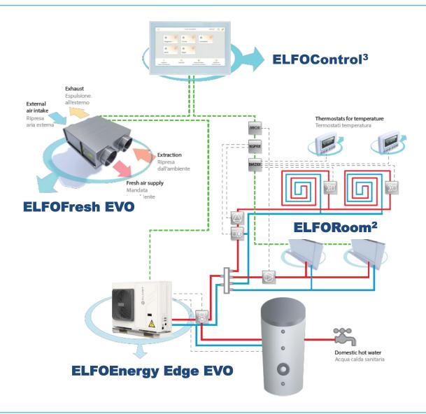
**ELFOControl**<sup>3</sup> is the advanced control system to manage the operation of the entire system.
