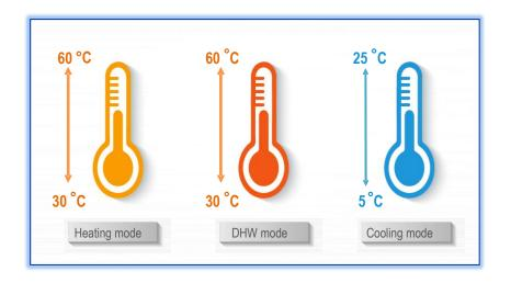
\* The leaving water temperature range will differ when setting different mode.
