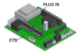
RS 485 Communication serial port with ModBus protocol (optional) Allowed the connection to supervisor system, or manage a small network up to 8 unit (one as master and 7 slaves)
