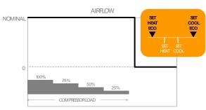
Variable airflow rate: supply airflow varies depending on the thermal load up to a minimum compatible value with distribution system. 40% of Airflow reduction → 70% energy savings
