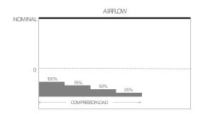
• ECO mode: airflow supply remains constant at varied thermal loads and is shutdown when the load is full filled
