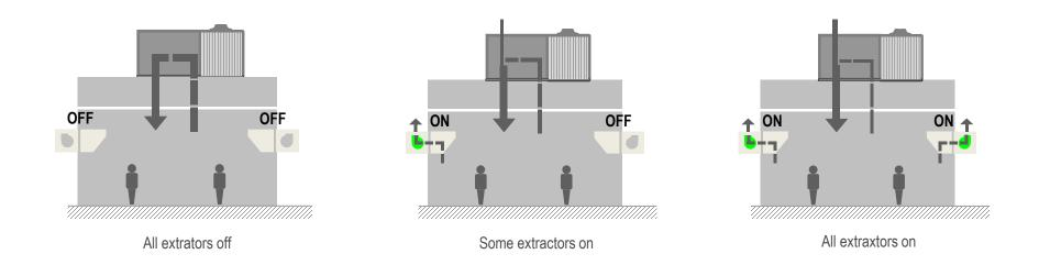
When the extractor hoods are activated the unit manage the fresh air damper to compensate the extraction air
